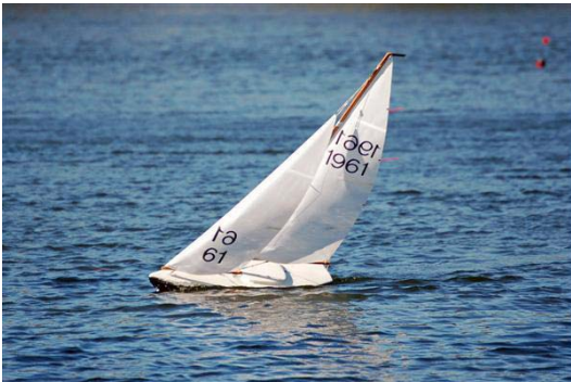
Soling 1 Meter 1961, built by Tom Willings of Florida. This boat is perfectly trimmed, with the main and jib leeches parallel (identical "twist"), and the speed shows it. Note the telltales on the leech of the mainsail- both streaming aft showing that the air is "attached" to the sail through the whole width of the sail. Thanks to Tom and Victor Model Products for the great picture!!!
