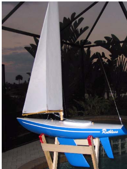
Soling 1 Meter 1961, built by Tom Willings of Florida. This boat is perfectly trimmed, with the main and jib leeches parallel (identical "twist"), and the speed shows it. Note the telltales on the leech of the mainsail- both streaming aft showing that the air is "attached" to the sail through the whole width of the sail. Thanks to Tom and Victor Model Products for the great picture!!!
